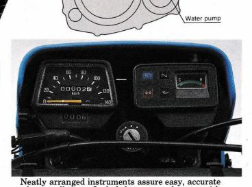
readout at all times. Included are a speedometer with
