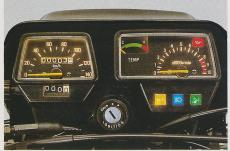
Although the liquid-cooled engine is virtually unburstable, there is still a full range of instruments which enable the rider to monitor its efforts. The angled-back instrument panel includes a tachometer and water temperature gauge as well as a speedometer and warning lights. It is protected by the neat headlamp fairing.
