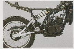
The Monocross rear suspension has a box-section rear sub-frame triangulated for total rigidity. Its movement is controlled by a single De Carbon-type shock absorber with gas/oil damping and a progressively wound coil spring. The more the compression, the more the spring resists it.
