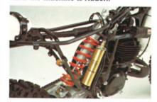
To match the increased engine performance, the new rear mono cross suspension helps to lower the centre of gravity of the YZ 490 for 1983 and
