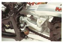
ments. The front fork has been improved with the use of a valve on the foot of the fork legs which regulates the damping characteristics on the compression side. A new rear mono cross suspension, a lower centre of gravity, and an overall weight reduction make the steering and handling of the YZ 250 LC even better than before! We will not be surprised to see the new YZ 250 LC leading the field
