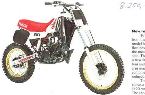
The 1982 YZ 80 LC which has so successfully dominated its class through-out the 1982 season with its impressive race performance has been improved for the new year, 1983. Taking its successful predecessor as a basis for further technical development and refinement, the 1983 YZ 80 LC's improvements are mainly centred on stability, steering and a more flexible engine characteristic.
