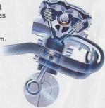
ide-Branch Exhaust Pipe This new exhaust system combines a main exhaust pipe with a side branch to improve torque at mid rpm range. The pulsation pressure generated in the exhaust pipe has generally adversely affected exhaust efficiency. In the new exhaust system, the exhaust gas expelled from the exhaust port is initially forced into the side branch, and when the exhaust valve is closed, the gas in the side branch is released through the main exhaust pipe. Consequently there is no drawback
