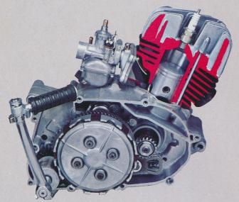
Yamaha's famous Torque Induction reed valve system gives the DT50M engine the flexibility of bikes three times its size and this, plus the five speed gearbox make the bike a zipply little performer on tarmac or trail. Reliability is ensured by the famous Yamaha Autolube system that feeds oil into the engine under pressure via a pump controlled by the throttle. The engine gets exactly the amount of oil necessary at any given speed.
