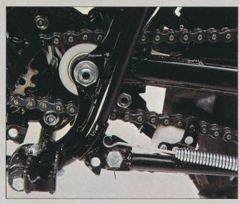
**Spring-loaded chain tensioner** helps to maintain an even chain tension and perfect adjustment even under extreme conditions.
