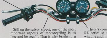
There's complete instrumentation on the RD series so that the rider knows exactly what he and his machine are doing. Speedometer and rev-counter plus oil level warning, neutral indicator and turn signal operating lights.
