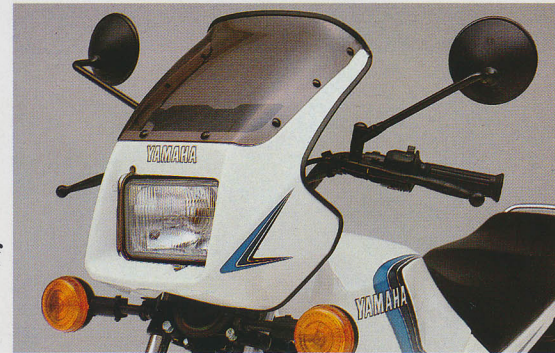
Shapely headlamp cowl is one of the results of relentless wind-tunnel tests. Square headlamp and highly visible turn indicators are employed for safe, fast riding.
