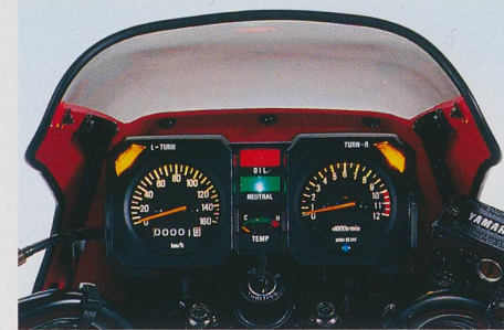
Speedometer, tachometer, temperature gauge, warning lights — the RD125LC is equipped with a full range of accurate, easy-to-read instruments. The ignition switch incorporates a safety steering lock position.
