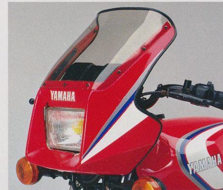
The shapely headlamp cowl is one of the results of relentless wind-tunnel tests. Square headlamp and highly visible turn indicators are employed for safe, fast riding.
