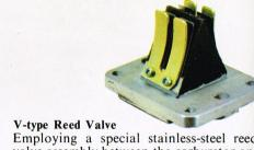
Employing a special stainless-steel reedvalve assembly between the carburetor and the engine, intake is positive and efficient. Operating due to pressure variations within the engine itself, the reed valves open and close on demand positively fueling the engine and preventing blow-back through the carburetor, resulting in increased torque
