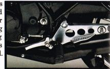
Cast aluminium plates act both as heel stoppers and to protect legs from the high-rise mufflers. Rear suspension is YAMAHA's all-conquering Monoshock. A triangulated rear sub-frame carries the wheel, which is suspended by a long spring-and-shock-absorber unit running under the tank to the steering head. The system provides not only rear wheel travel, but more positive damping, which allows the wheel to follow more closely the variations in road surface.
