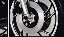
The wheels are YAMAHA Italic design, cast in alloy and finished in silver and matt black. The brakes are double disc front and waterproof, dustproof drum rear.
