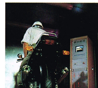
FAR LEFT All engines are tested and functions checked using a computer controlled facility.
