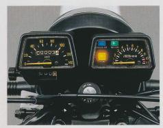
The instrument panel is steeply angled to give easy reading and includes a speedometer and tachometer, plus a full range of warning lights. The main ignition switch incorporates a steering lock for extra
