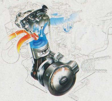
• Efficient 4-valve cylinder head, pentroof combustion chamber and YDIS guarantee plenty of power with miserly fuel consumption. Electronic CD ignition and automatic compression release give effortless starting, while the counter balancer smoothes out vibration.
