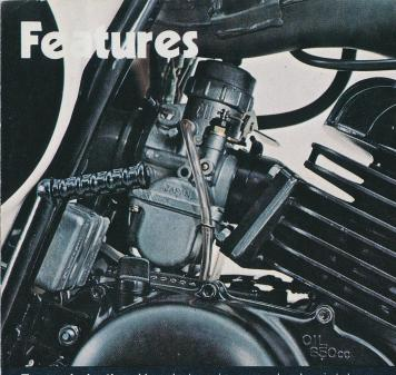
**Torque Induction**, Yamaha's unique reed-valve intake system, feeds the engine the exact mixture of fuel and air it needs. The result is more horsepower, particularly at low rpm's.
