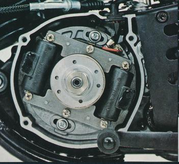
**C.D.I.** ignition generates a hotter, more even spark and helps reduce spark plug fouling. Gone are the conventional breaker points and all the problems associated with them.
