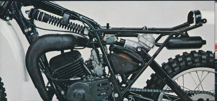
New Monocross® suspension, the same as used on Yamaha's National and International MX winners, allows 7.1" of rear wheel travel. This longer stroke insures more traction by soaking up bumps and helps keep the rear wheel and power on the ground.
