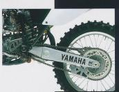
Rear suspension/Shock Fully adjustable fade-resistant shock is worked by a lightweight YZ250-type aluminium swinging arm to give superb handling and traction — and with low-friction needle roller bearings, smooth action is assured.
