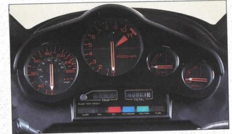
Businesslike instrument panel features electronic tach, speedometer, coolant temperature gauge and fuel gauge.
