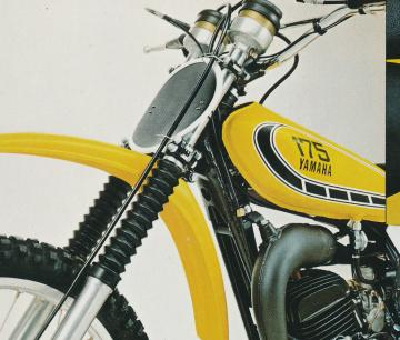
Yamaha's exclusive air cushioned front forks soak up sharp jolts without bottoming. Lightweight alloy rims and conical hubs minimize unsprung weight.
