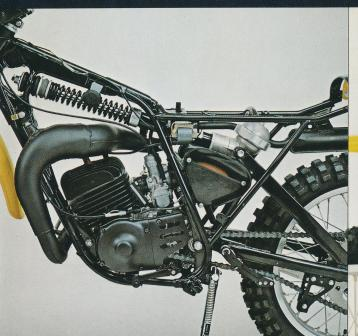
New Monocross® suspension, the same as used on Yamaha's National and International MX winners, allows 7.1" of rear wheel travel. This longer stroke insures more traction by soaking up bumps and helps keep the rear wheel and power on the ground.
