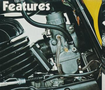
**Torque Induction**, Yamaha's unique reed-valve intake system, feeds the engine the exact mixture of fuel and air it needs. The result is more horsepower, particularly at low rpm's.
