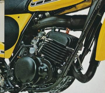
**Double loop frame** creates a low center of gravity for better balance. For extra comfort and handling ease, the exhaust system is tucked out of the way under the padded saddle.
