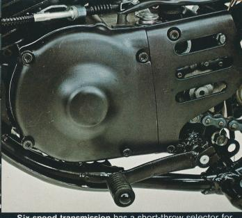
**Six-speed transmission** has a short-throw selector for quick, positive shifts. The close ratio helps keep you close to the peak power band.
