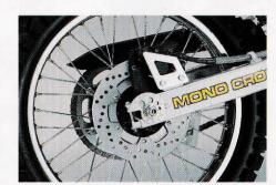
The 230mm front brake disc is drilled to dissipate heat, while the 220mm rear disc uses the same caliper and master cylinder as our YZ motocross racers.
