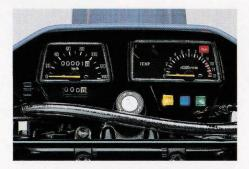
The DT125R instrument panel is neatly mounted behind a small head fairing. Panel contains speedometer, rev-counter and resettable trip meter.
