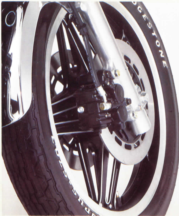
NEW DUAL-PISTON CALIPERS GRIP SLOTTED BRAKE DISCS.
