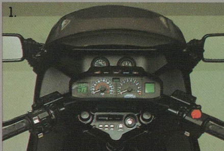
1. VF750S: Sport fairing instrument panel holds voltmeter and altimeter.
