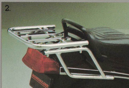
2. VF750S: Trim, chrome-plated luggage rack matches the looks of the machine.
