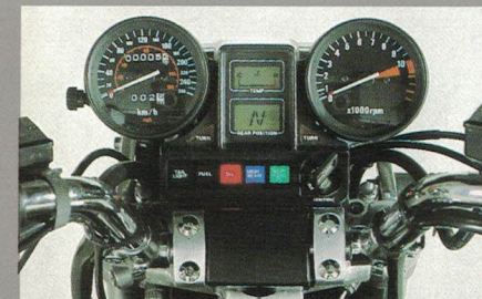
INSTRUMENTS INCLUDE DIGITAL GEAR POSITION AND FUEL STATUS INDICATORS. HANDLEBARS ARE INDIVIDUALLY ADJUSTABLE.
