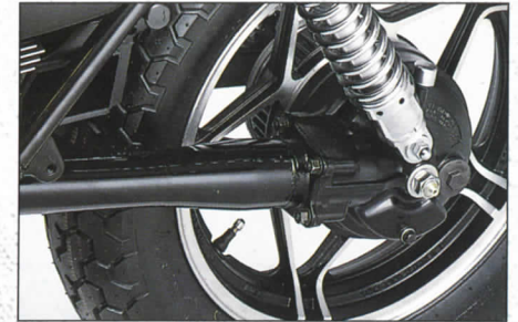
Twin shocks with two-stage damping bolt to an extra-long drive- shaft that reduces up-and-down torque reaction.
