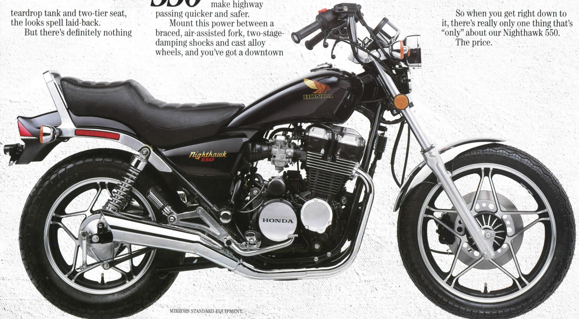
Twin shocks with two-stage damping bolt to an extra-long drive- shaft that reduces up-and-down torque reaction.
