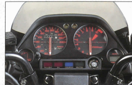
Attractive instrumentation includes electronic tachometer, fuel gauge and LCD gear position indicator.
