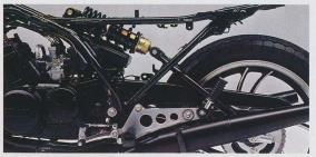
Good suspension is vital for a fast sports motorcycle, and that is why Yamaha use their race-proven Monocross suspension on the RD350LC. The De Carbon type suspension unit allows five settings, so the suspension can be set up to suit each individual rider and varying loads or road conditions.
