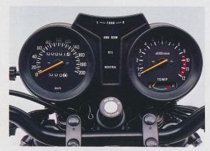
All the information you need can be obtained at a glance from the centrally mounted instrument console. Alongside the easy to read rev-counter and speedometer are a full range of warning lights and engine temperature gauge. The speedometer incorporates a trip indicator.
