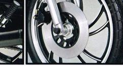
The wheels are YAMAHA Italic design, cast in alloy and finished in silver and matt black. The brakes are single disc front and waterproof, dustproof drum rear.
