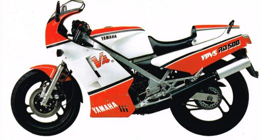
The Yamaha RD500LC uses the world's first (and so far, *only*) liquid-cooled vee-four, two-stroke power unit in a volume production motorcycle. It closely follows the layout of the Grand Prix 500 racer developed by three-time World Champion, Kenny Roberts, and taken to another world title for Yamaha in 1984 by Eddie Lawson.
