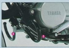
4 Foot-peg guards (patent pending) For added protection under severe operating conditions, guards were installed low on the machine to protect the brake pedal, shift lever and the rider's feet from injury due to rocks and other obstacles.
