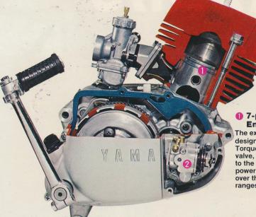
1 7-port Torque Induction Engine (Patented)
