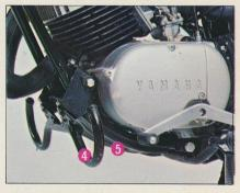
Foot-peg guards (patent pending) For added protection under severe operating conditions, guards were installed low on the machine to protect the brake pedal, shift lever and the rider's feet from injury due to rocks and other obstacles.
