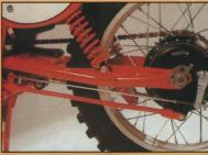
2. A good part of Qualifier's easy handling is due to light weight, especially unsprung weight. Magnesium hub is one reason. A new chromoly swingarm is another. It not only starts
