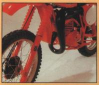
1. Qualifier's excellent handling starts with an utterly rigid 4130 chromoly frame. Our lightweight cantilevered Can-Am MX design positions the engine for lowest center of gravity. To maintain handling character-
