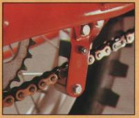
quide set-up is as foolproof as they come, yet perfectly simple. The roller tensioner and the one-piece wraparound block in the rugged chain quard are both made from
