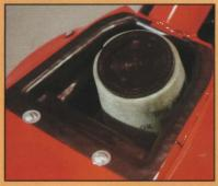
5. This new Qualifier air intake has been carefully designed to keep engine air clean and dry. The K&N filter is equipped with an additional foam envelope. The airbox is sealed to provide only a single rear entry
