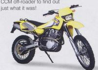
The 604DS shares the same engine & frame as the R30, along with practical unpainted bodywork. It has a longer swing arm allowing a quick wheel change, easily converting from Supermoto to trail bike. This flexibility is reflected by over half of CCM customers choosing a second set of wheels when they purchase.
