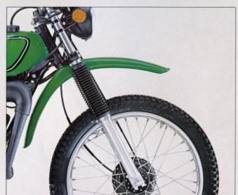
Heavy-duty front forks have increased travel for easier handling and a more positive feel when riding over obstacles and road hazards. New YZ-type rubber covers protect the mechanism.
