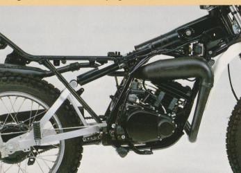
(Chassis: 2) The longer travel and the slower action of the monoshock suspension allows the rear wheel to follow the irregularities of the terrain, rather than bouncing over them. The ride is easier, progress faster, and maximum power is delivered to the ground. The rigid sub-frame keeps the wheel in alignment, minimizes weaving, and assists positive steering in the rough and on the road.
