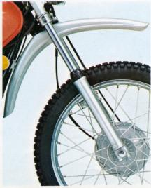
Front forks and high-rise front fender Designed to absorb a wide variation of shocks and vibration, the enduro front forks help reduce rider fatigue while maintaining maximum stability. These forks have a long stroke enabling comfort plus maneuverability for all types of road or trail travel, and the high-rise front fender is durable and installed so that the front wheel will not clog with mud or brush.
