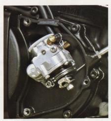
Continuously monitoring the rotational speed of the engine and the throttle opening, Autolube precisely controls the amount of oil, from a separate tank, to be mixed with the gasoline. This automatic gasoline and oil mixing system, which was developed by YAMAHA, improves engine operation by maintaining optimum performance under all rid-
