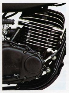
With lighter piston and connecting rod material plus a radial head-fin design, the large 2-stroke engine has less vibration, less noise and better heat dissipating characteristics.
