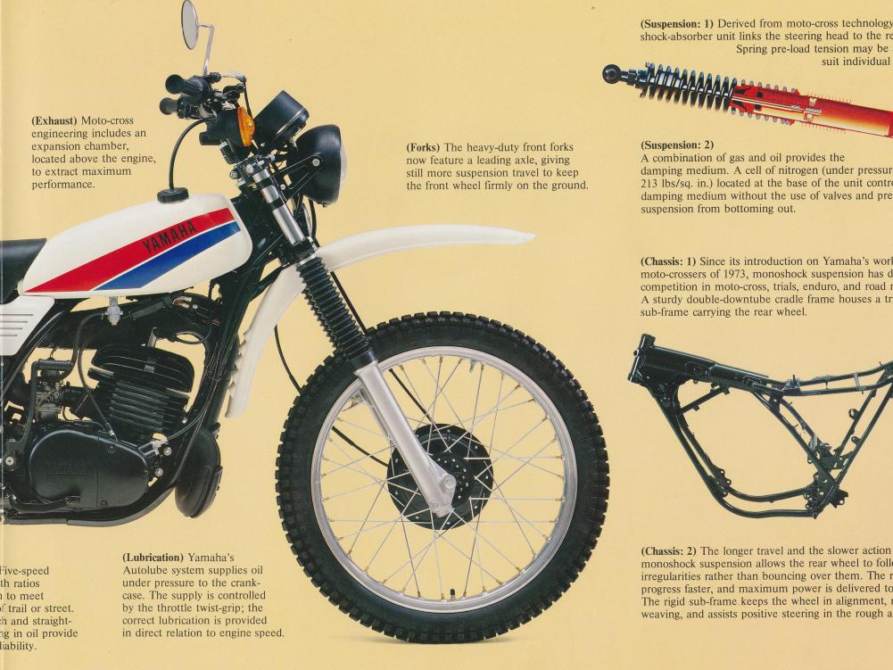
(Suspension: 1) Derived from moto-cross technology, a single shock-absorber unit links the steering head to the rear sub-frame. Spring pre-load tension may be adjusted to suit individual rider.
