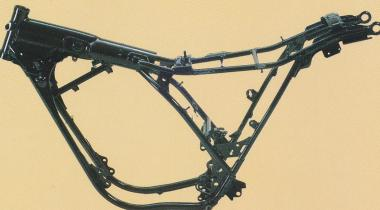
(Chassis: 2) The longer travel and the slower action of the monoshock suspension allows the rear wheel to follow surface irregularities rather than bouncing over them. The ride is easier, progress faster, and maximum power is delivered to the ground. The rigid sub-frame keeps the wheel in alignment, minimizes weaving, and assists positive steering in the rough and on the road.
