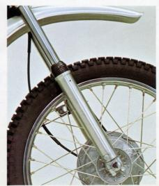
Front forks and high-rise front fender Designed to absorb a wide variation of shocks and vibration, the enduro front forks help reduce rider fatigue while maintaining maximum stability. These forks have a long stroke enabling comfort plus maneuverability for all types of road or trail travel, and the high-rise front fender is durable and installed so that the front wheel will not clog with mud or brush.
