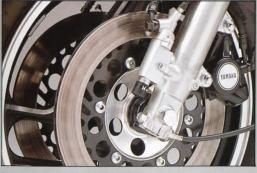
The dual front discs are internally ventilated, just like those on Formula One race cars, for maximum fade-resistant operation under even extreme use. And the anti-dive mechanism helps keep the bike level during hard braking, thus maintaining balance and control while entering a corner.
