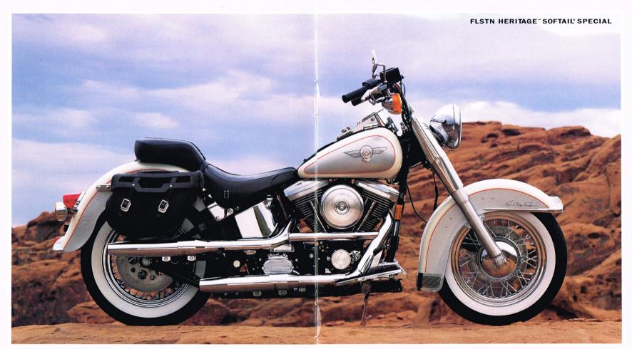
Chrome fishtail mufflers; shotgun-style exhaust, chrome laced wheels, floorboards, wide whitewall tires, silver and white two-tone paint, forged copper and fired enamel Fat Boy\*-style tank emblem, cowhide inserts
