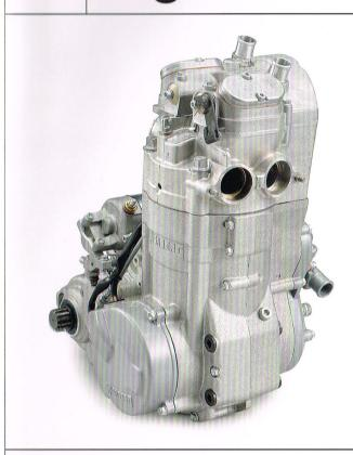
Compact and light construction with deep centre of gravity; width under 260mm; high performance camshaft; reinforced valve cover for increased number of revolutions; water pump in the clutch cover; water pump driven by the crank shafts revolutions for optimal cooling.
