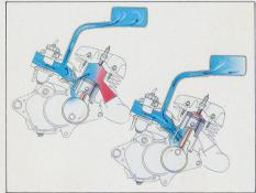
The exclusive Yamaha Energy Induction System (YEIS) consists of a small chamber connected to the intake manifold. This chamber acts to dampen and otherwise absorb fluctuations in intake tract pressure and mixture velocity. In so doing, it evens out the air flow, resulting in better combustion, and superior power, torque and response in the low- and mid-range bands—with less fuel consumption and no additional moving parts.
