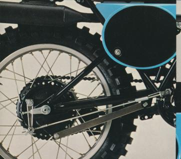
New Monocross<sup>®</sup> suspension, the same as used on Yamaha's National and International MX winners, allows 7½" of rear wheel travel. This longer stroke insures more traction by soaking up bumps and obstacles while keeping the rear wheel on the ground.
