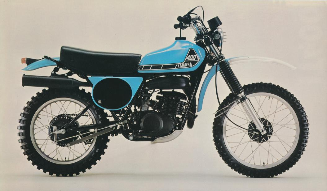
The IT400 is an all new off-road competition machine ideally equipped for International Trials events. Or you might simply call it a pure competition Enduro. It has the same powerful two-stroke single engine, double-loop frame and Monocross\* suspension as Yamaha's big-bore
