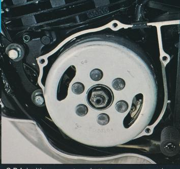
**C.D.I.** ignition generates a hotter, more even spark and helps prevent spark plug fouling. Gone are the conventional breaker points and all the problems associated with them.
