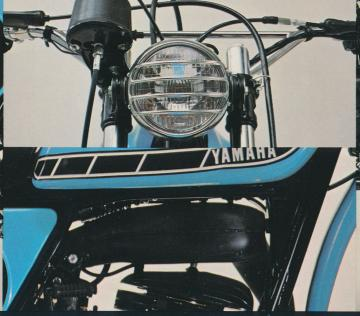
Off-road lighting kit and quiet exhaust system conform to requirements of International Trials events. The tuned silencing system reduces noise without affecting performance. It is center mounted for greater comfort and control.
