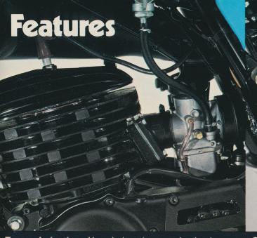
**Torque Induction**, Yamaha's unique reed-valve intake system, feeds the engine the exact mixture of fuel and air it needs. The result is more horsepower, particularly at low rpm's.
