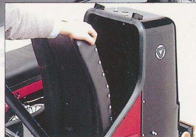
Storage compartment on Velorex side car
