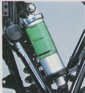
NEW DAMPING ADJUSTMENT - Standard on all 1984 motocross machines, gives extra adjustment to the Uni-Trak suspension.
