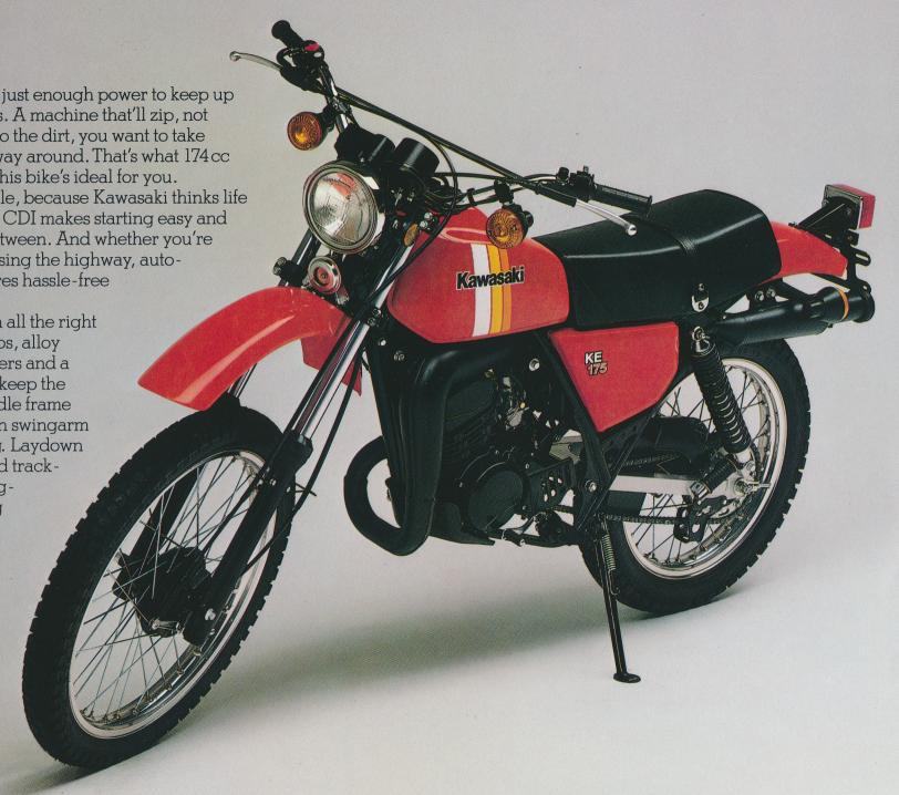
The KE175 has a rugged twostroke engine with Electrofusion cylinder, Superlube Injection and maintenance-free CDI ignition.
