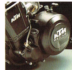
Modern art: Lighter, more compact engine casings without balancing shaft.
