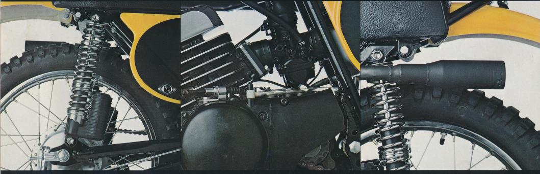
Thermal-Phase rear shocks have built-in oil coolers to prevent overheating, no matter how hard or long you ride. Interchangeable jets also allow you to adjust compression and rebound characteristics individually.
