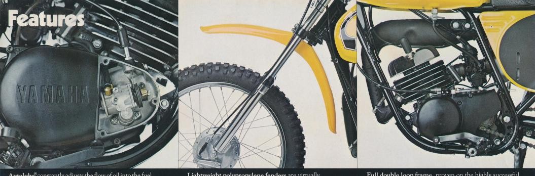
**Autolube**<sup>®</sup> constantly adjusts the flow of oil into the fuel mixture according to engine load and speed, resulting in increased engine life. For those who want to save a little weight and premix, the unit is easily detachable.
