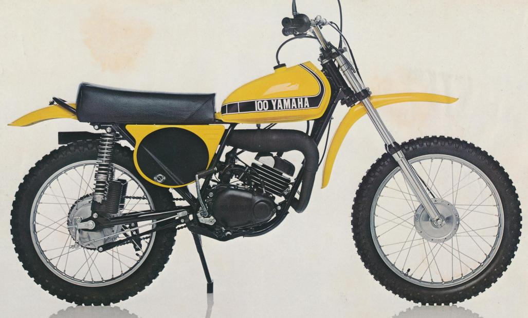
Like all the bikes in Yamaha's MX stable, the MX 100 has been completely redesigned for 1974. This year, it has a true motocross frame, with a much lower center of gravity. A new lightweight front hub. A new center muffler. Longer travel front forks. And Thermal-Phase
