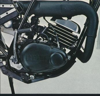
Full double loop frame, proven on the highly successful Yamaha factory motocrossers, cradles the engine lower, results in lower center of gravity, better steering geometry, and better handling.
