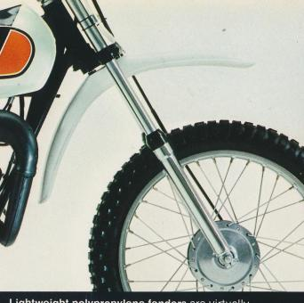
Lightweight polypropylene fenders are virtually unbreakable. Fiberglass seat assembly is also featherlight, but well padded. Conical hubs reduce unsprung weight without reducing braking efficiency.
