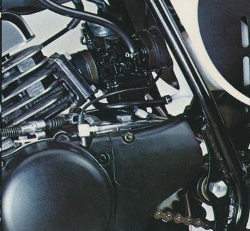
**Torque Induction,** Yamaha's unique intake system, utilizes a reed valve to feed the engine the exact amount of fuel and air it needs. The result is more <u>horsepower</u>, particularly at low rpm's.
