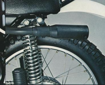
**Expansion chamber/silencer** design cuts down noise without cutting down power. Over-the-top configuration results in better road clearance, less chance of burns.
