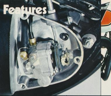
**Autolube**® constantly adjusts the flow of oil into the fuel mixture according to engine load and speed, resulting in increased engine life. For those who want to save a little weight and premix, the unit is easily detachable.
