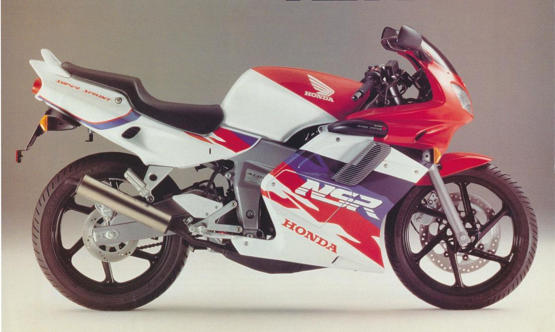
Unmatched Grand Prix styling of the new NSR125R-R sets the standard for learner legal motorcyclists. Never before has such a high-specification Honda been available to novice riders. With its sturdy aluminium Alcast Zeta frame, cast wheels, six-speed transmission, disc brakes, Pro-Link monoshock rear suspension and single-cylinder two-stroke engine with electronic exhaust valve, the NSR125R-R is an irresistible combination of technology and responsive handling.
