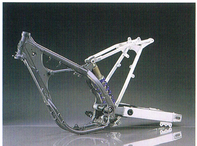
Round/box tubing frame (photo: RM250)
