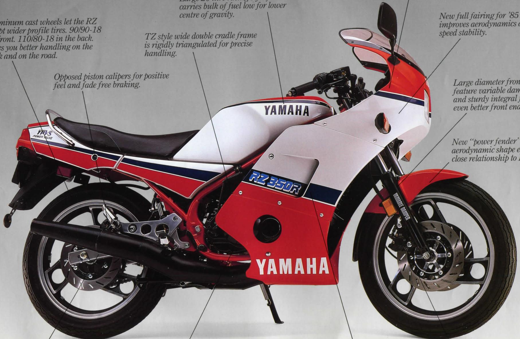
Improved swing arm design incorporates full length box section tubing for increased strength and needle bearing pivot for optimum compliance.
