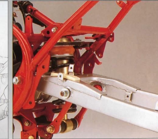
Square section steel frame employs a widely spaced double cradle design with hefty bracing at the steering head and swing arm pivot. The lower right frame section removes to allow easy engine access.
