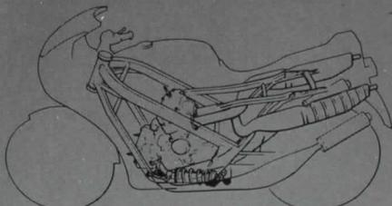
4 into 1 into 2 exhaust system follows exactly the same routing as YZR500 GrandPrix racer, permits an incredible 52 degree lean angle.
