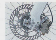
Semi-floating front disc with kevlar hose
