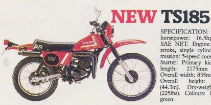
SPECIFICATION: Maximum horsepower: 16.5hp/5500rpm. SAE NET. Engine: 183cc. 2stroke, single cylinder. Transmission: 5-speed constant mesh. Starter: Primary kick. Overall length: 2175mm (85.6in). Overall width: 835mm (32.9in). Overall height: 1125mm (44.3in). Dry-weight: 102kg (225lbs). Colours: Red, blue, green.
