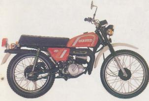
SPECIFICATION: Maximum horsepower: 2.92hp/6000rpm. SAE NET. Engine: 49cc. single cylinder, air cooled, 2stroke. Transmission: 5-speed constant mesh. Starter: Primary kick. Overall length: 1855mm (78.03in). Overall width: 775mm (30.51in). Overall height: 990mm (38.98in). Dryweight: 71kg (156.53lbs). Colours: Red, white, blue.
